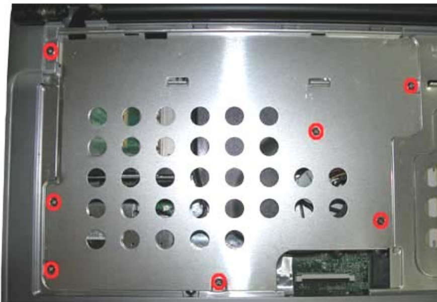
Fig. 20 Removing the screws retaining Heat Plate
